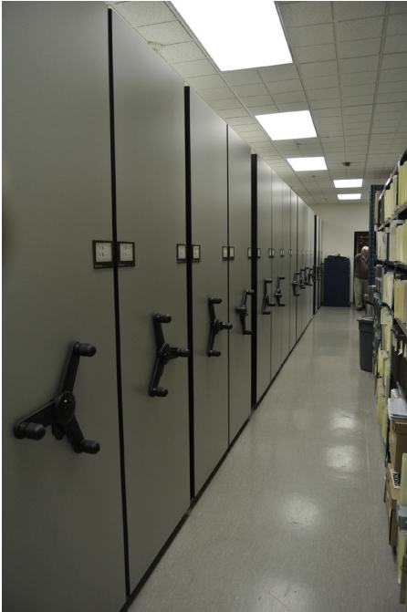
Part of the Archives' stacks, showing rolling shelving used for storage of textual and graphic records.
